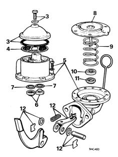
If the valves are renewed, ensure that they are fitted to operate in the correct directions and staked in.
