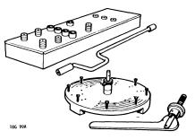
18G 99 A Clutch Assembly Gauging Fixture
