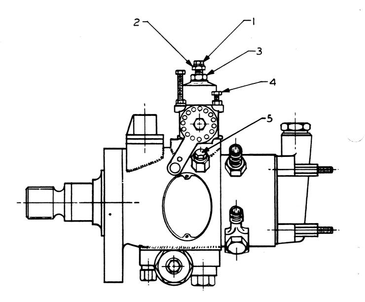
On all prewired engines dating from early 1975 onwards bleed screw (#5) has been relocated to the opposite side of the fuel injection pump.
