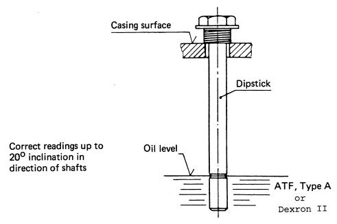
To check the oil level, just insert the dipstick, do not screw in. Retighten the hex screw with the dipstick after the oil level check.
