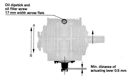
The position of the cover plate underneath the actuating lever is factory-adjusted to ensure equal lever travel from neutral position to A and B.
