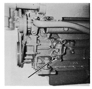
Typical Mechanical Fuel Lift Pump
